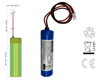
Lithium- Battery Pack with a protection electronics (PCM single cell monitoring), Protects the battery against overcharge, deep discharge and short circuit.
